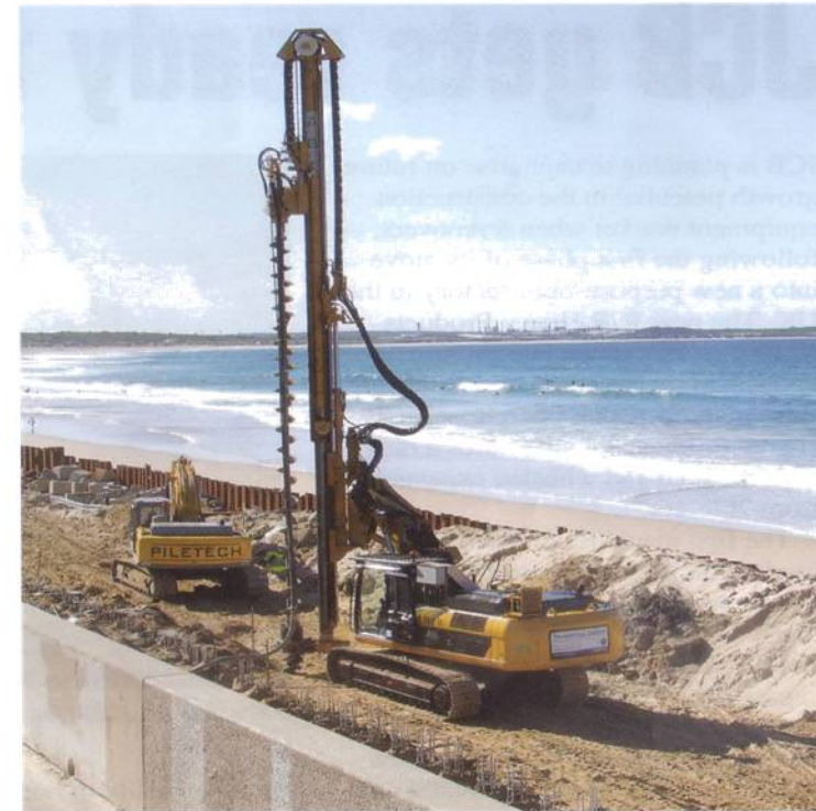
The ABI Mobilram TM 13/16 features high torque, telescopic mast and stable base unit.
